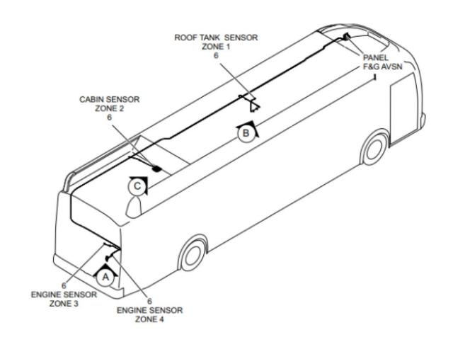
Monitors 6 Zones for Compressed Natural Gas Leaks and Engine Fires
